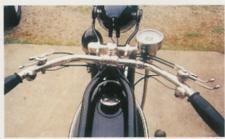
The single carburetor is rather primitive, controlled by two levers on the top, right of the handlebar. There is a third lever on the top, left of the handlebar.
