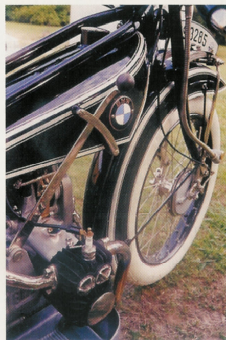
The R32 has a hand-shift with two neutrals (one between first and second gear and another between second and third gear).
